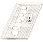
Use chemical process monitors suitable for steam autoclaves/sterilizers at the indicated cycle temperatures and times in or on each package or load being sterilized.
