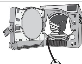
Inspect and clean the three chamber filters.
